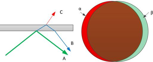
Figure 14. Projected areas on diffuser for smaller L distance between sensors
