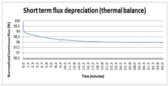
Fig 1. Flux depreciation due to the thermal balance
