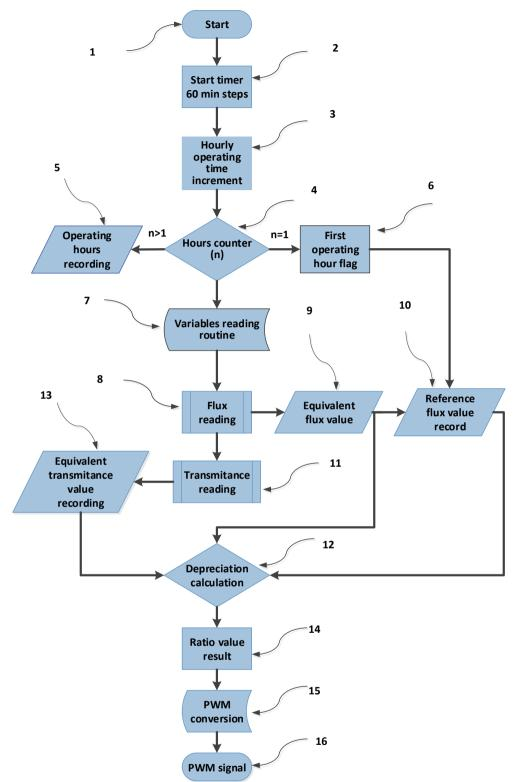
Figure 15. Flow diagram of the BLO process
