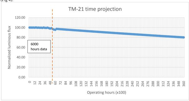
Otherwise, the results estimate an 80.23% depreciation level for luminous flux after 36 000 hours operating time (Fig 4).
