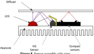
Figure 8. Sensor assembly side view.
