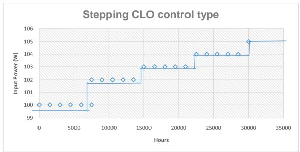
Figure 6. Example of stepping of CLO control type
