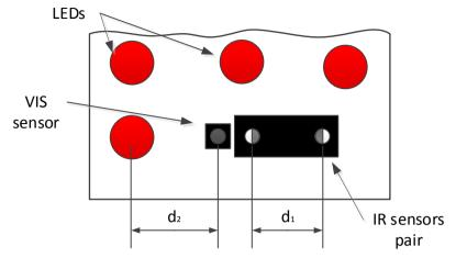
Figure 10. Sensors assembly top view
